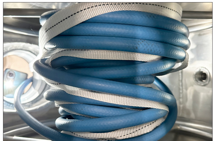
8. Wind the hose and brake band together in the drum
