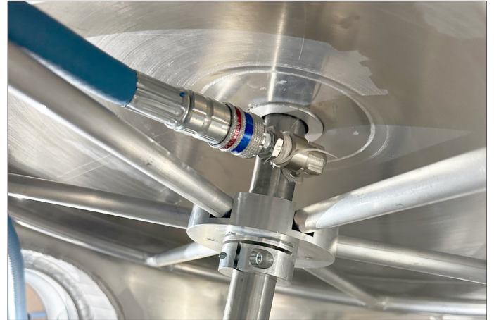
6. Connect the air hose to the fitting
