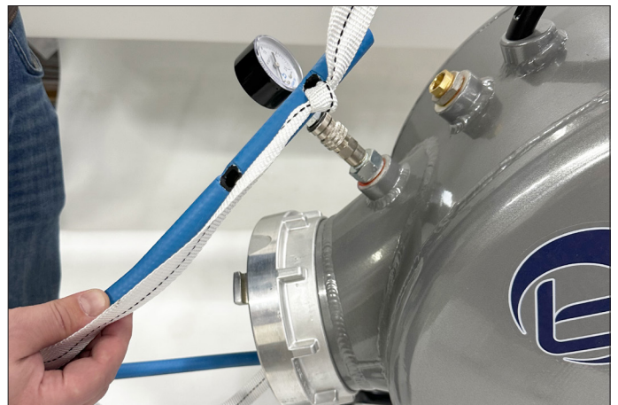
11. Tie a brake band through the hole so that you can put it in the knot of an open-end hose or a calibration hose
