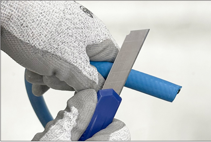
9. Cut holes in the hose in the same place on both sides
