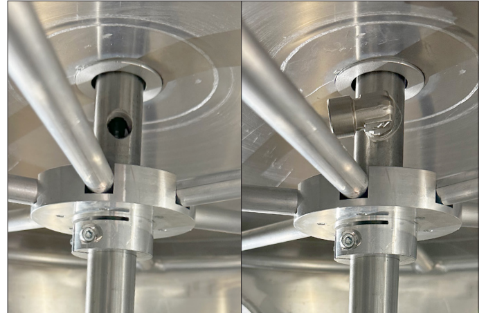
4. Connect the pipe elbow fitting onto the joint on the shaft inside the drum
