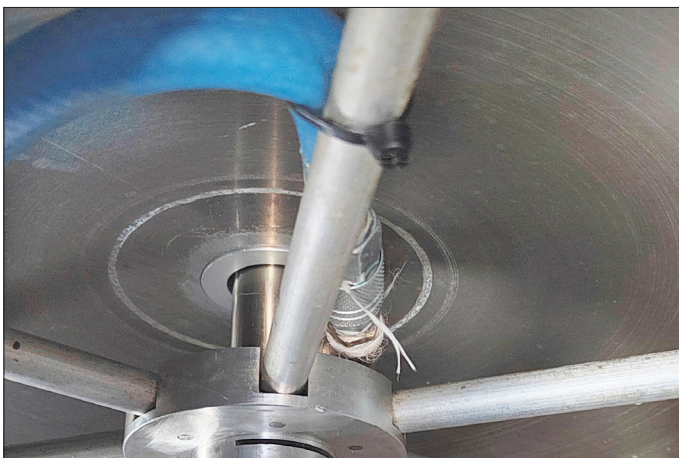
7. Fasten the air hose to the bar with a cable tie
